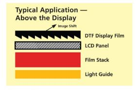
**Figure 3** shows the DTF located on top of the LCD.
