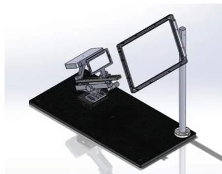
Figure 2. Solid model of a Luminit HUD demo - There are no lenses between the diffuser and the combiner hologram because all optical functions are in the volume of the hologram on a surface relief structure and embedded in an automotive windshield.
