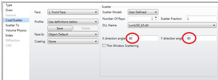
Since the formulas and algorithms are already imbedded, there is little additional effort needed to change the modeled diffuser's output characteristics. For the user, it is two simple entries of the desired X and Y spread angle.
