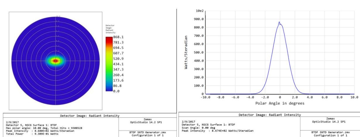
**$1^\circ$  Diffuser profile with 1/18 degree resolution**
