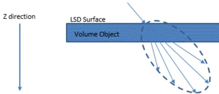
Since this is a random statistical model, each ray that strikes the surface will take a different path to exit, even if it has the same exact path in. The LSD model scatters the rays in such a way as to emulate the shape of the statistical distribution of the Luminit LSD.
