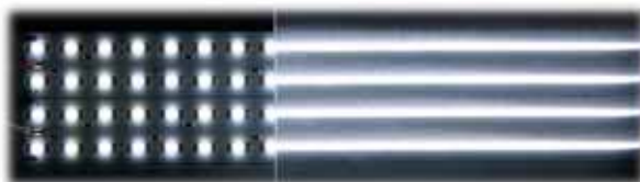
LED panel with 60° x 1° diffuser
